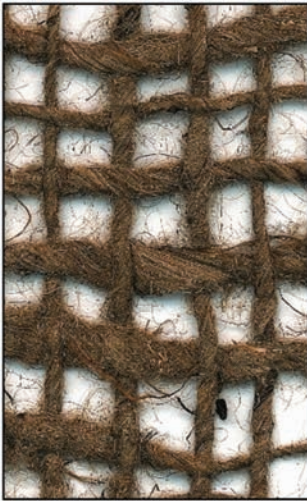
Fig 3: A close-up view of common jute net that can be used as a form of anti-erosion mat on a gentle slope.
